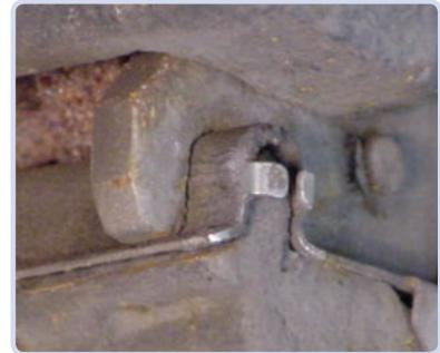
Caliper/Pad/Guide Rust Buildup From Lack of Lubrication
